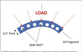
SolidCasy Polymer's QOR-TEC technology could make polymer concrete segments a viable and longer-lasting alternative to traditional ones.
